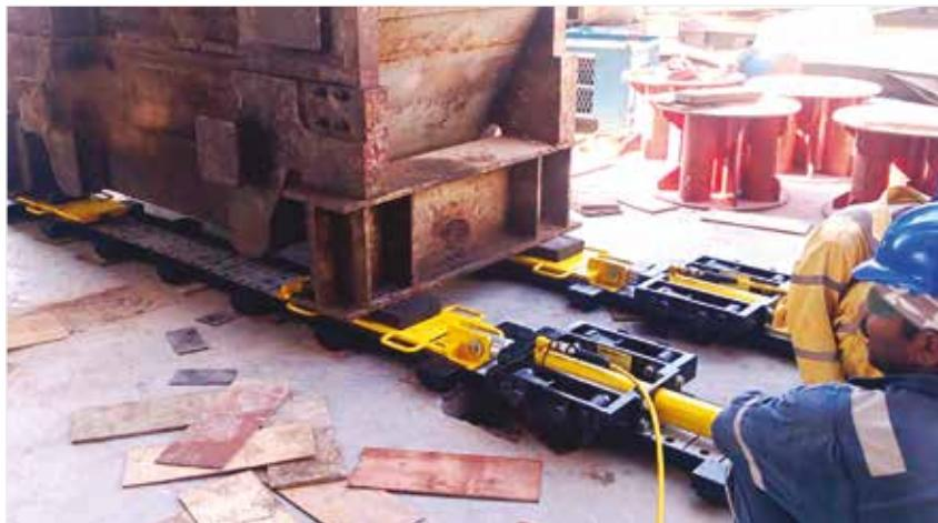
▼ LH400 Skidding used to remove an old press from a facility to make room for new equipment.
