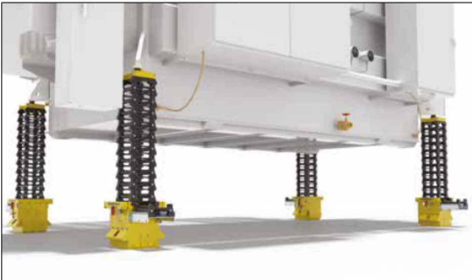
▼ Typical set-up with 4 Self-Locking Cube Jacks and cribbing blocks to lift a transformer. Enerpac recommends to power the Cube Jack using SFP-Series Split-Flow Pump (pump and hoses not shown).
